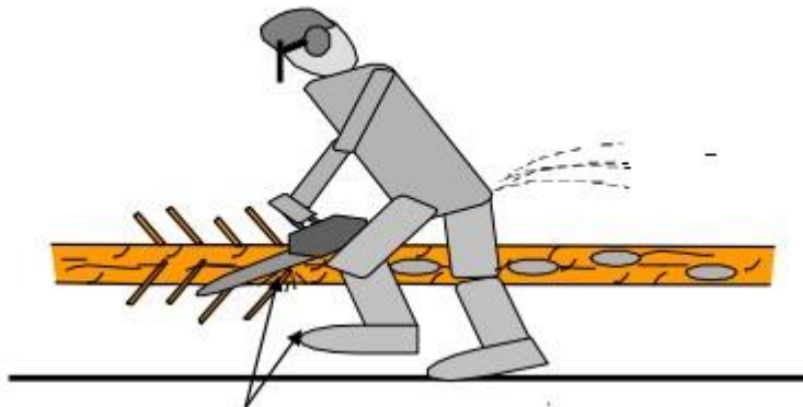
Fig. 44: Incorrect movement during limbing (walking)
